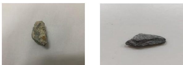
(a) Recycled aggregate (b) Natural aggregate Fig. 1 – Picture of RA and natural aggregate
